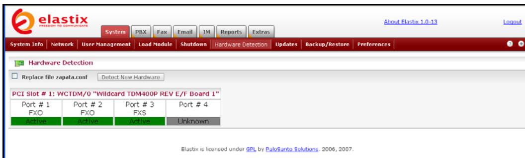
A400P with 2 FXO and 1 FXS modules installed
