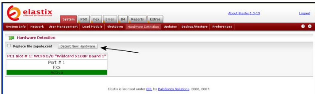
A100P card installed
