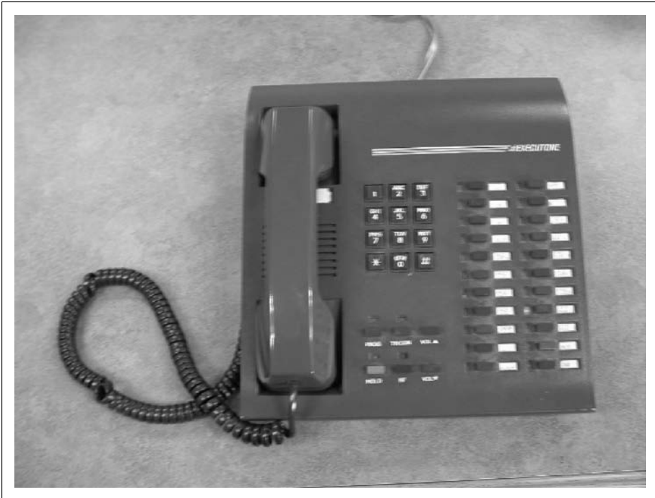
Figure 4-10. Traditional digital business phones like this one are a part of the PBX system's TDM bus
