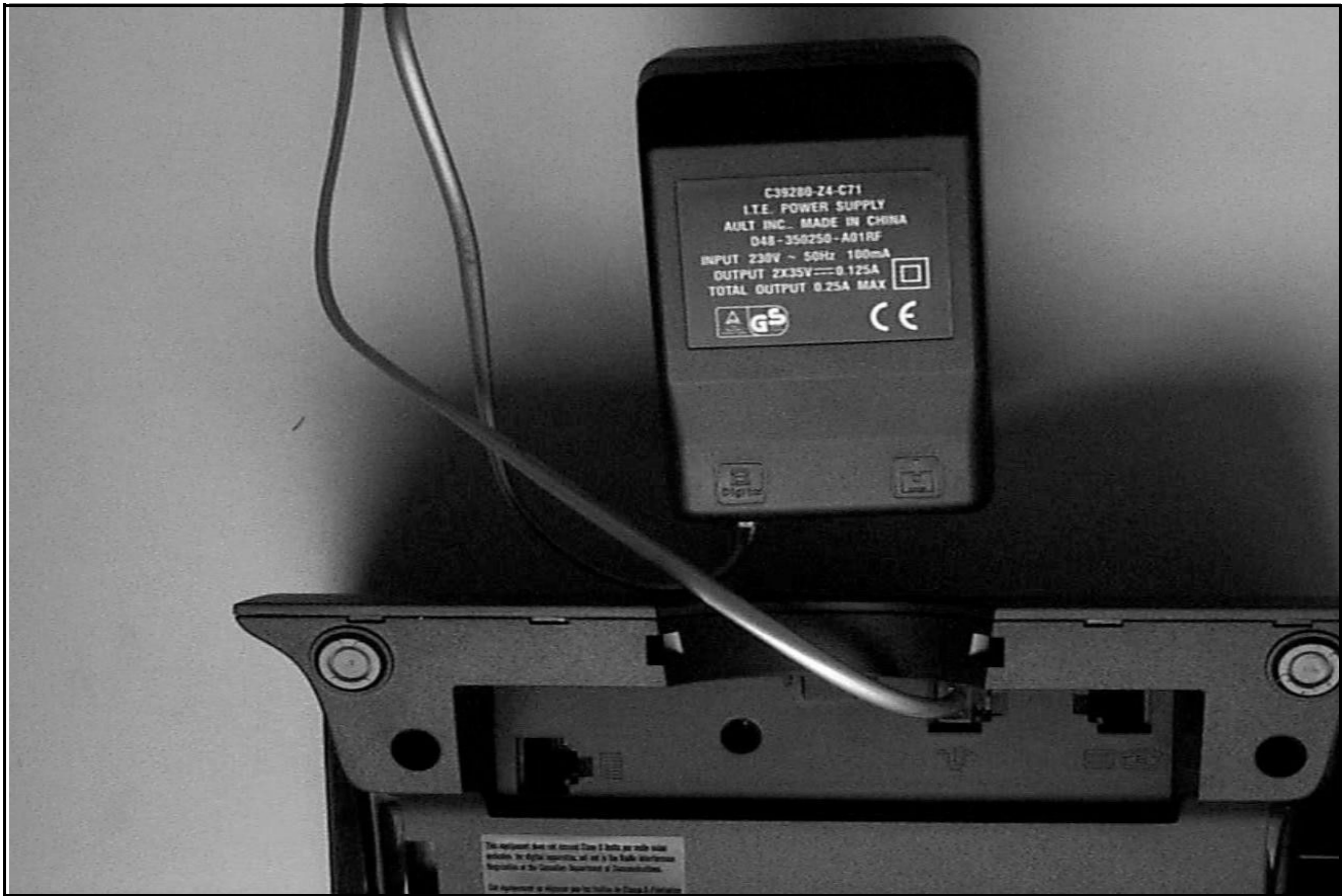
Figure 2-6 Power supply to BLF
